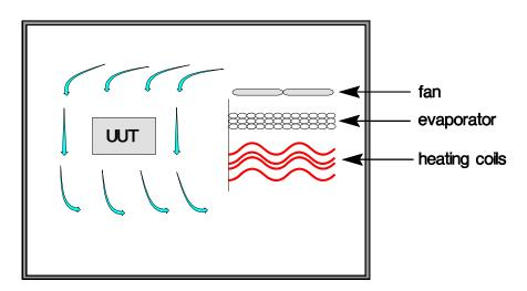
Figure 3 – Single zone chamber layout
