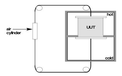
Figure 4 – Two zone air-to-air chamber
