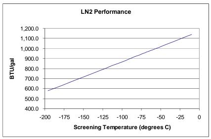
Figure 6 – LN2 Performance for various screening temperatures
