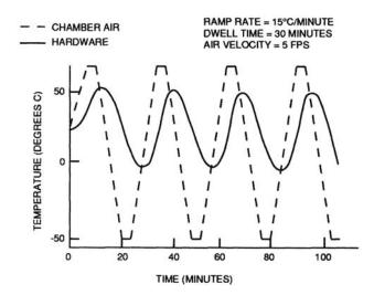
Figure 1 – Product response for the low airflow case
