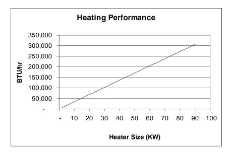
Figure 7 – Heating Performance for various heater sizes
